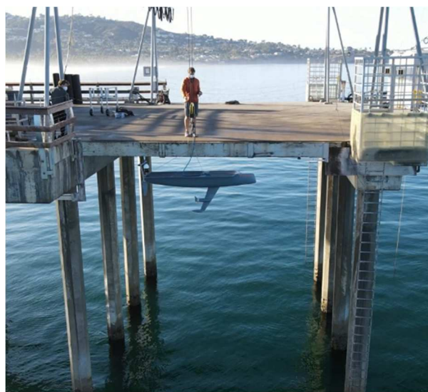
Figure 1. X3 Crane Launch & Recovery off Scripps Pier, La Jolla CA
